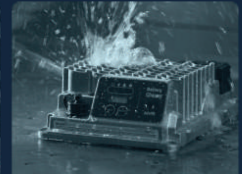
Water Ingress Testing
